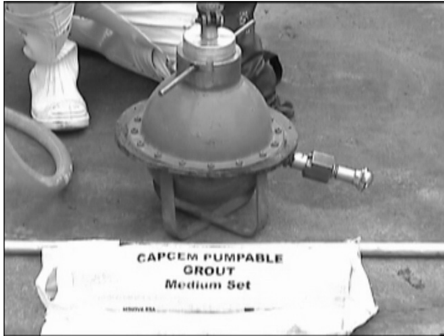
Figure 10. Minova's Spudnik® Pump.
